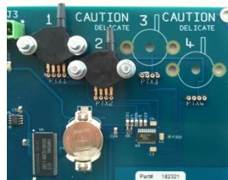
1-4 Channels on the same Circuit Board
